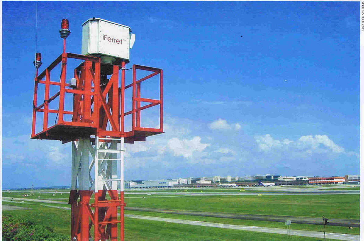
iFerret in service at Changi. The FOD detector is on pilot trial at Chicago's O'Hare International Airport.
